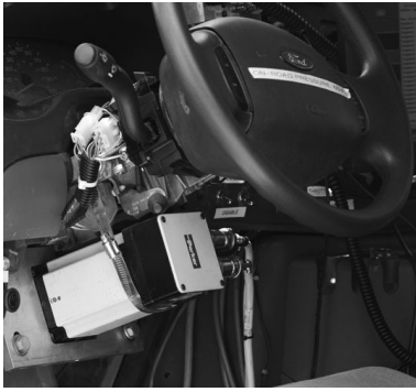
Fig. 2. Photograph showing Alice's power steering assembly.
