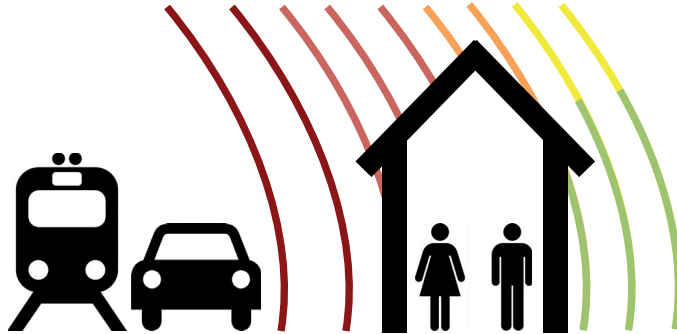
Figure 3: The concept of quiet side, where one side is sheltered from traffic noise
