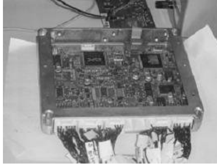
Figure 3.17 Engine Control Unit with the embedded controller software.
