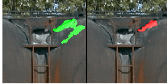
Fig. 11. (1.9 MB) Simultaneous imaging of ammonia and ethylene leaks showing the isolation of the ammonia flow using the gas-correlation technique. Measurement conditions: Time 17:25, Air temperature 19.2 °C, Surface temperature 31.5 °C, Relative humidity 50 %, Ammonia gas flow 15 l/min, Ethylene gas flow 10 l/min, ZnSe gas cell with ammonia 1 atm., Filter: Spectrogon LP9200.
