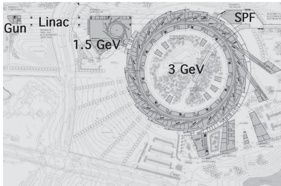
Figure 1: Overview of the MAX IV facility. The gun bunker is at the top left followed by the underground linac tunnel. The 1.5 GeV and 3 GeV storage ring buildings are indicated. The short-pulse facility (SPF) is indicated at the top right.
