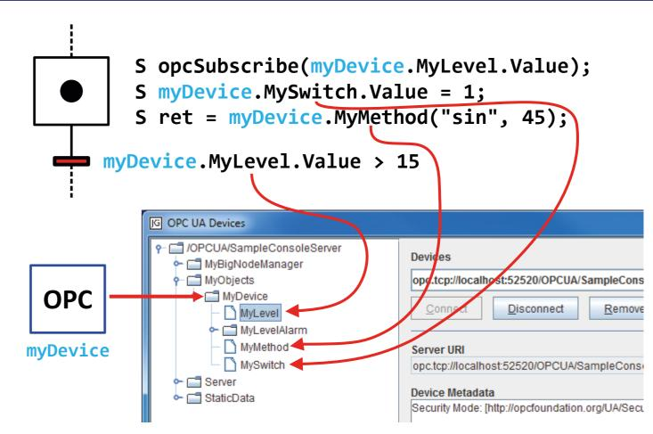
An *OPC UA Object* is bound to a node in an OPC UA server. The OPC UA variables and methods are then used like native variables and methods.
