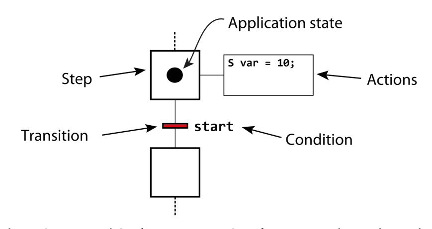
Grafchart is a graphical programming language based on the PLC standard language SFC. The basic building blocks are steps (application states) with actions (what to do when) and transitions (how and when to change application state).
