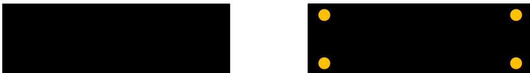
Figure 3. Example of layout of amber flashing lights in the corners of a TIS (zero lights on the left image and 4 lights on the right image).
