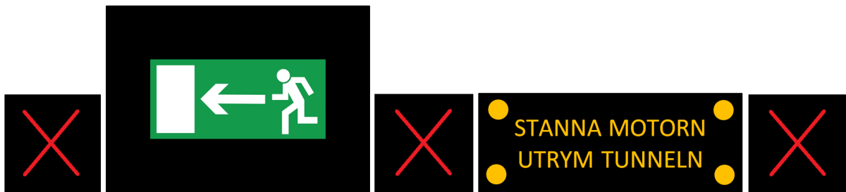
Figure 16. Recommended TIS design.
