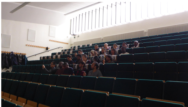
Fig. 4. Nine active users surrounded by eleven non-active users (crowd) at UE site MS 1. MS antennas are being held vertically and describe random trajectories.
