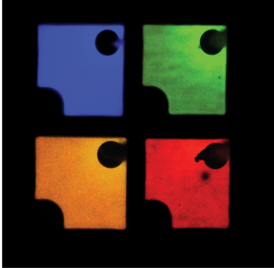
Figure 1.6: GaN nanowire LEDs made by GLO AB, emitting in the blue, green, amber and red wavelength regions.
