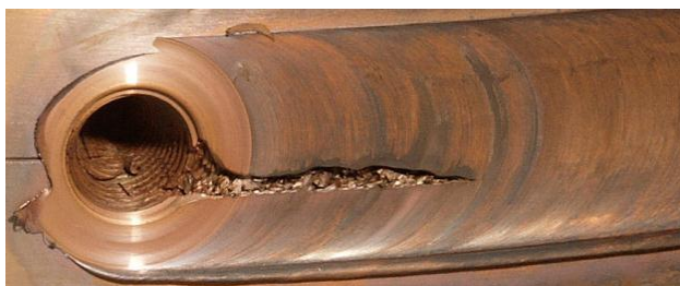
Figure 4-1. Visible wormhole during lid weld at TWI.
