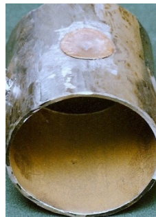
Fig. 8 Result of welding with detonator on a pipe with a hole
