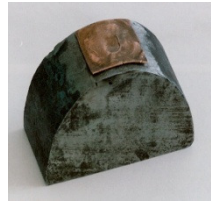
Fig. 7 Result of welding with detonator on a curve shape
