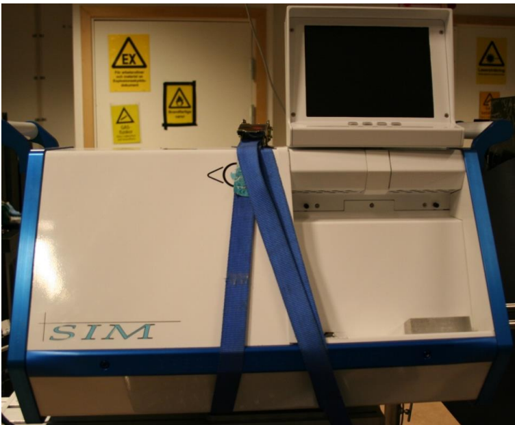
Figure 2.2 A photograph of the SIM 8 framing camera.
