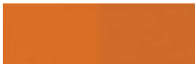
Figure 5. Visual comparison of an unexposed film and an exposed (47 mGy), shown side-by-side where the exposed film is shown to the right.
