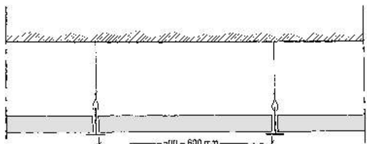
Fig. 42 Flat roof consisting of two layers of woodwool slabs. Space is left in the top layer for reinforced concrete beams. These beams and the concrete slab are cast at the same time. The under layer of woodwool slab breaks the thermal bridges created by the concrete beams. The ceiling can either be left as it is, which gives good sound absorption, or plastered. (Using 30 and 120 mm thick woodwool slabs gives a U-value of 0.5 W/m 2 K).
