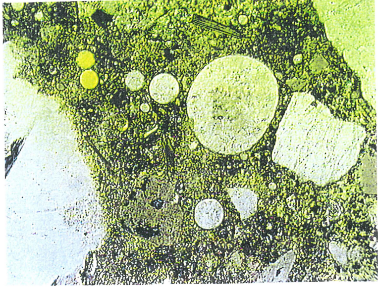
Picture 1. A picture of concrete specimen in transmitted light in thin section. A few empty air voids and typical "round aggregates" in the completely filled air void system. The size of the photographed area is about 0.8 mm x 1.3 mm.
