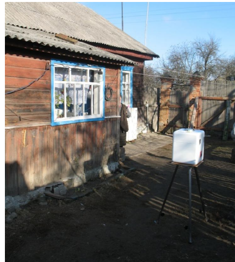
Fig. 2. In situ measurement of the ambient dose rate in a garden in the village of Svetilovichi.
