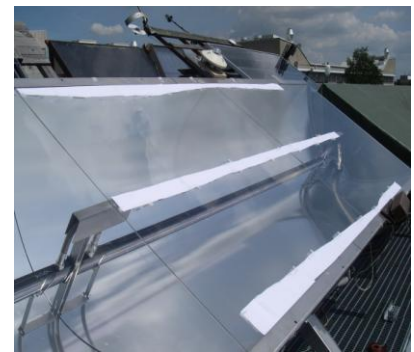
Fig. 5. Areas covered with paper where the incident light is not focused on the PV cells.
