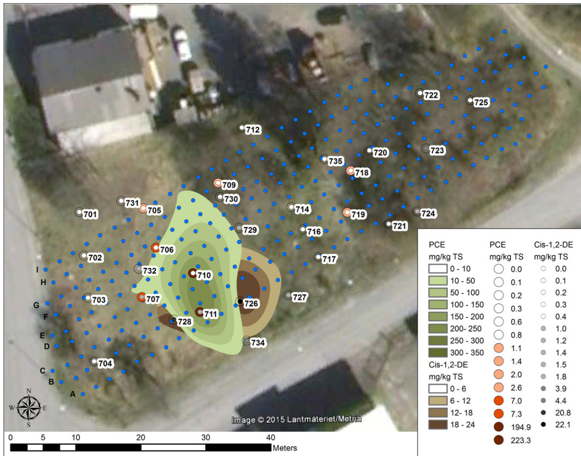
Fig. 3. Summarizing results from the chemical analyses of soil samples taken in the sandy chalk till (below – 4 mamsl). The interpolated PCE surface show approximately the main location of the source contamination, while the interpolated Cis-1,2-DE surface indicate the main degradation zone.
