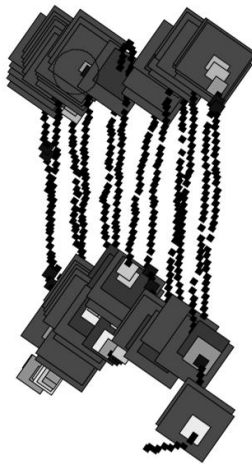
Fig. 2. An approximately 70×100 m 2 schoolyard in the village of Starie Vyshkov (2013). The size of the squares indicate the 137 Cs activity (larger squares is equal to higher activity). Variations in the straight walking lines are mainly caused by the precision of the GPS-signal.
