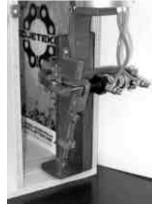
Figure 4.27 The book gripper grasping a book in a compartment in the bookshelf.
