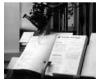
Figure 4.31 The end-effector has opened the book and the finger of the readerboard is holding it open.
