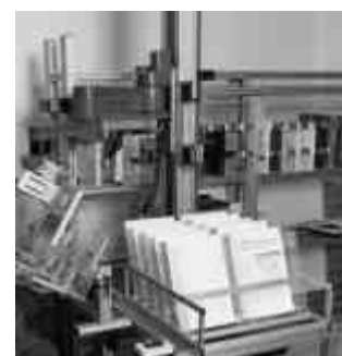
Figure 4.44 The RAID2 can lift a book from the readerboard very carefully because the movable thumb of the end-effector grasps the front of the book.
