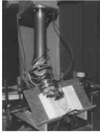
Figure 4.30 Various turning movements were tested. The end-effector is rotated while turning a page.
