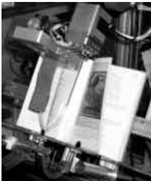
Figure 4.52 When the robot turns a page, the page-turning gripper carries out a circular movement. The brush on the lower edge of the gripper stops the subsequent page from turning. In this position, the finger of the gripper is moved towards the book.
