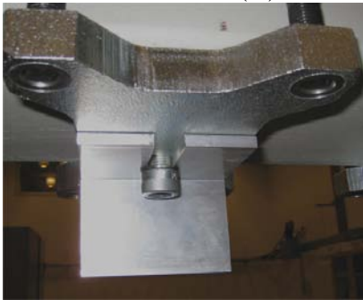
Figure 3 - The top brackets can be moved in two degrees of freedom.
