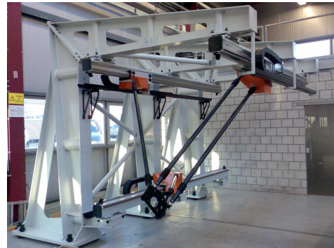
Fig. 1. Full size Gantry-Tau prototype (SMERobot TM project)
