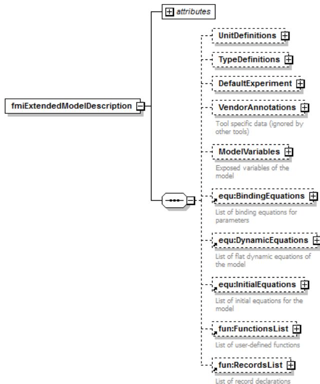
Figure 2. Overall structure of the DAE XML schema
