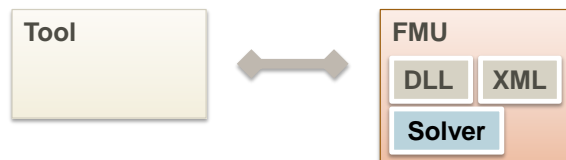
Figure 3: Overview of a co-simulation FMU, note that the solver in this case is within the FMU.
