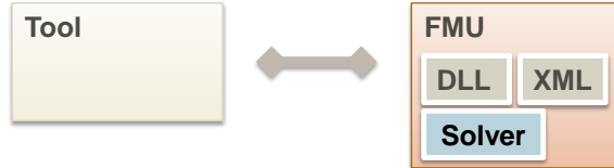
Figure 4: A co-simulation FMU and the connection to a tool for simulation. Note that the solver is inside the FMU.
