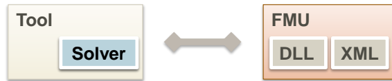
Figure 2: Overview of a model exchange FMU, note that an external solver is required by the tool in order to solve the model.
