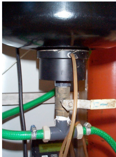
Figure 5.6 Close-up view of the special cup, which is used together with the on-line instrument Evita from Danfoss.
