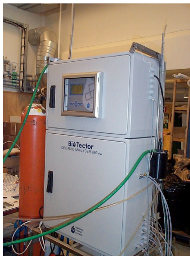
Figure 3.1 On-line instrument for analysis of TOC.
