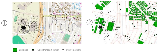
Fig. 10. Example of one user's trajectory projected on: (1) OpenStreetMap raster layer and (2) Vector layer retrieved from our geo-database.
