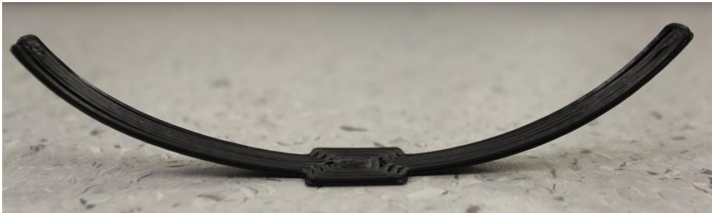
Figure 8, 3d printed sample showing exaggerated shrinkage effect
