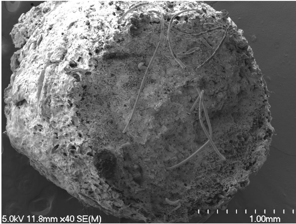
Figure 22, 30 wt% harakeke filament fracture surface showing polyester fibres
