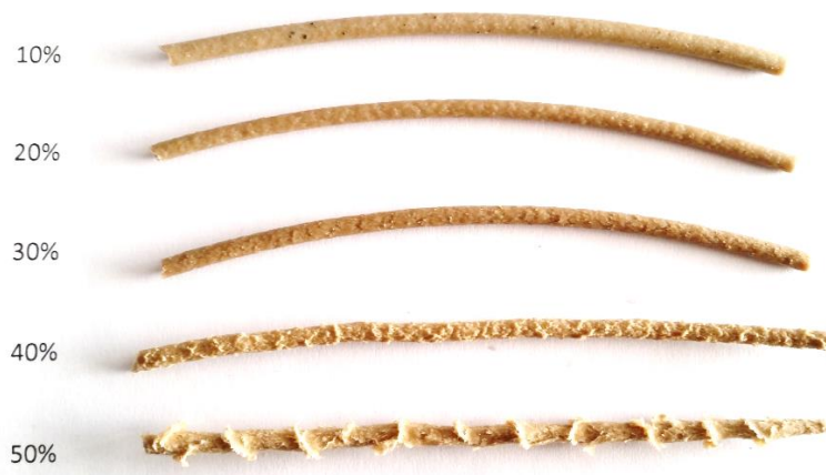
Figure 11, Influence of fibre content on surface finish
