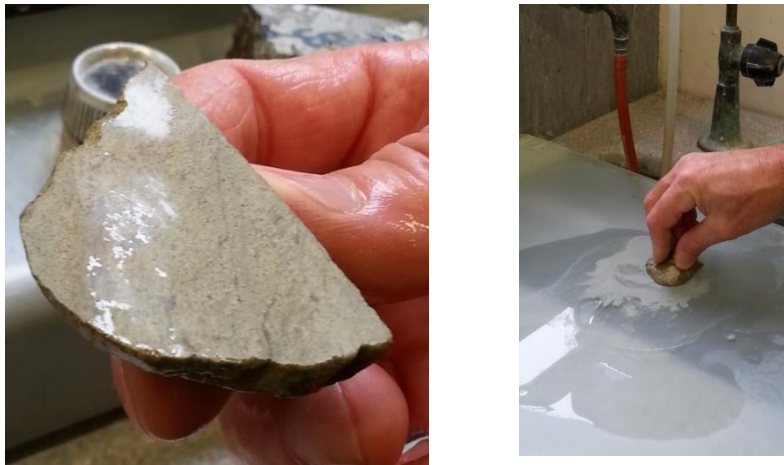
Figure 3.11. Excess resin is ground off using a slurry of grinding powder and water, so that an even coating of resin is visible on the surface.
