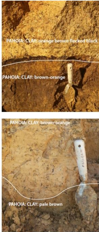
Figure 4.10. Stratigraphic log and photos of SS1, Bramley Drive, Omokoroa.
