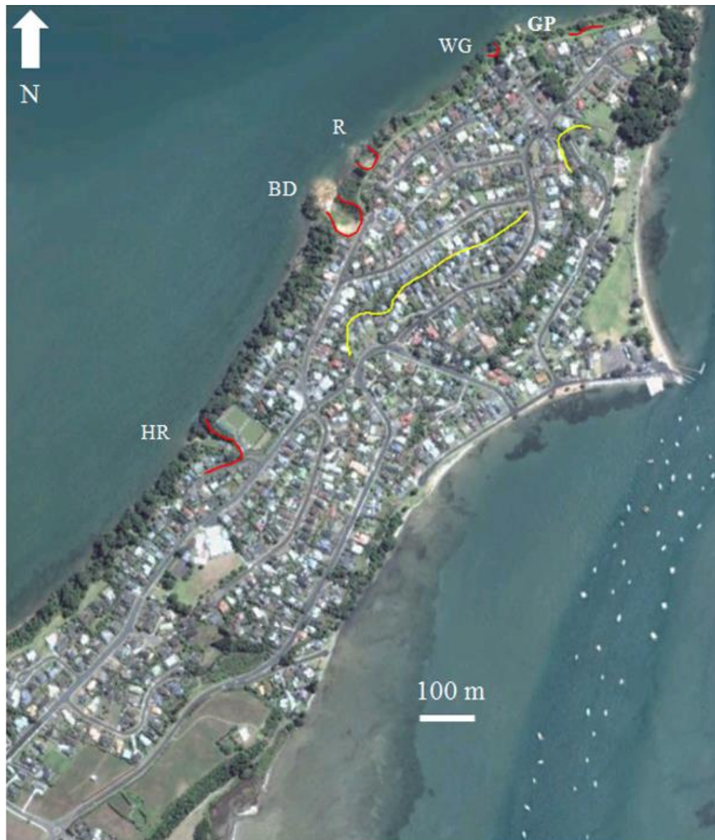
Figure 4.2. An aerial view of Omokoroa (2015, GoogleEarth), and respective landslide scarp locations. Historic landslides, including Bramley Drive (BD), Ruamoana Place (R), Hamurana Place (HP), Walnut Grove (WG), and Gerard Place (GP) are outlined in red. Inferred relict landslip scarps are outlined in yellow, after Christophers (2015).
