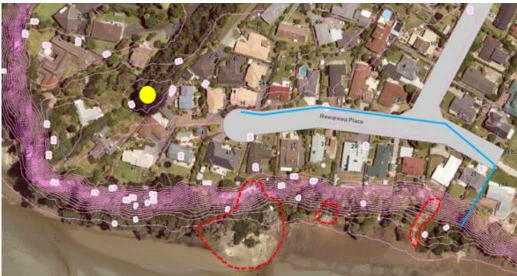
Figure 4.12. Aerial photo taken in 2015 of the south side of Matua Peninsula, with overlain 1 m contours. Several landslides occurred following heavy rainfall in 2012 (red outline), including the largest one studied in this thesis. Storm water drains at the eastern end of Rewarewa Place, as outlined in blue. The yellow circle indicates the peak at 23 m. Photo: http://gismob.tauranga.govt.nz/
