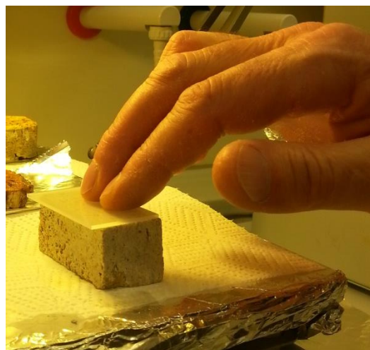
Figure 3.12. The frosted slide was out face down and moved in a circular motion to remove air bubbles between the sample and the slide.
