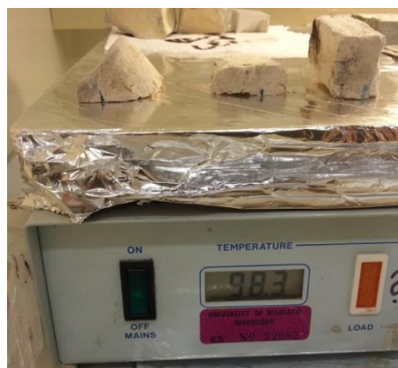
Figure 3.9. The dried block heating up on the hot plate prior to impregnation of resin. Heat allows the resin to permeate deeper into the sample.
