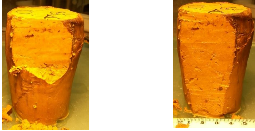
Figure 3.8. Omokoroa (240 kPa) post-failure, showing the cut failure surface exposing the shear zone.
