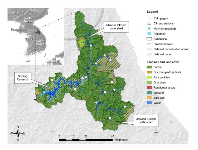
**Figure 3.1** Location and land use and land cover classification of the Soyang Reservoir watershed including subbasin configuration and climate and monitoring stations required for the hydrological modeling with SWAT. The Mandae and Jawoon Stream watersheds are the two major agricultural production "hotspots" mainly responsible for water quality degradation of the Soyang Reservoir (Arnhold et al., 2014; Park et al., 2010).
