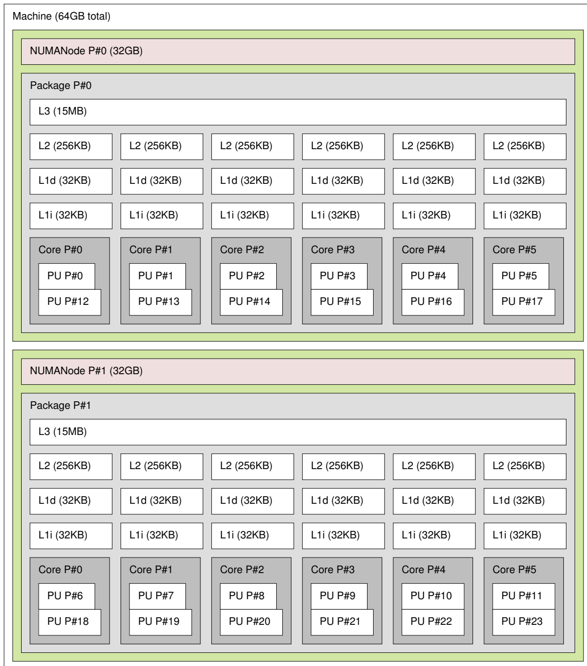
Figure A.1: Processor topology of the 24-thread Intel Xeon system.
