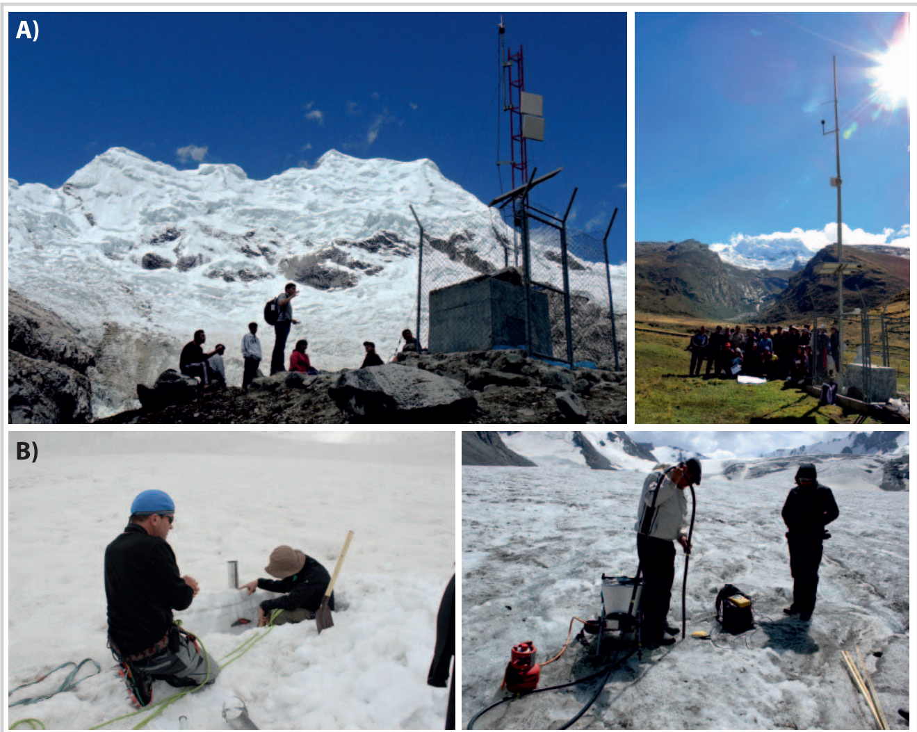
FIGURE 3 (A) Monitoring stations in the Cordillera Blanca of Peru, where potential ice and rock-ice avalanches into Lake 513 constitute a serious danger for downstream communities, including the city of Carhuaz. The rapidly changing glaciers can also exacerbate the hazard situation (Photos provided by N. Salzmann, 18.9./7.10.2013); (B) In situ mass balance measurements: determination of the accumulation (left) and ablation (right) at Golubin glacier in the Tien Shan, Kyrgyzstan. (Photos provided by M. Hoelzle, 13./14.8.2012).
