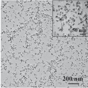
Fig. 4. TEM images of commercial Chemicell fluidMAG-D SPIONs.
