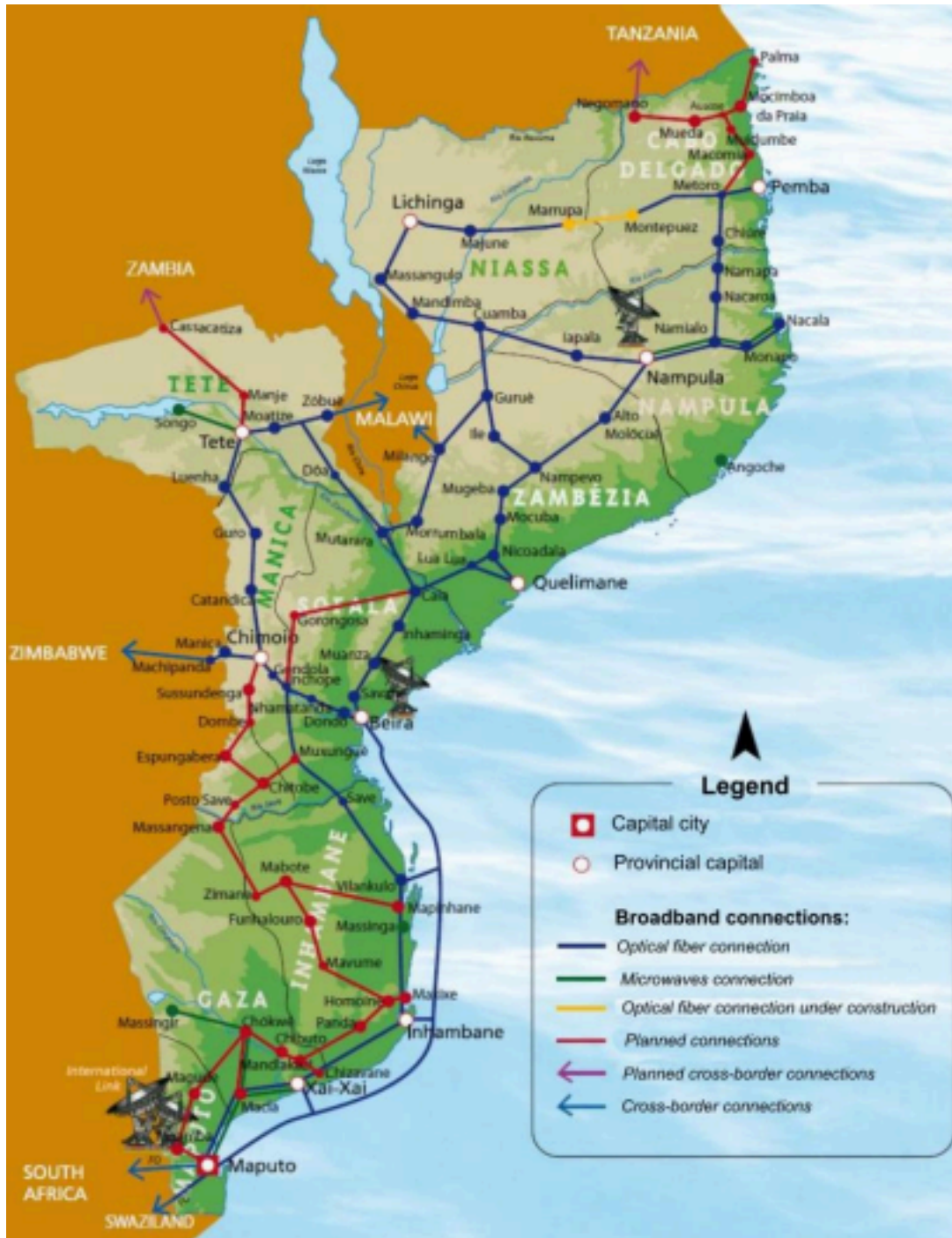
Figure 2:6 TDM Existing and planned fiber links (Source: TDM and Accenture study http://www.oafrica.com )
