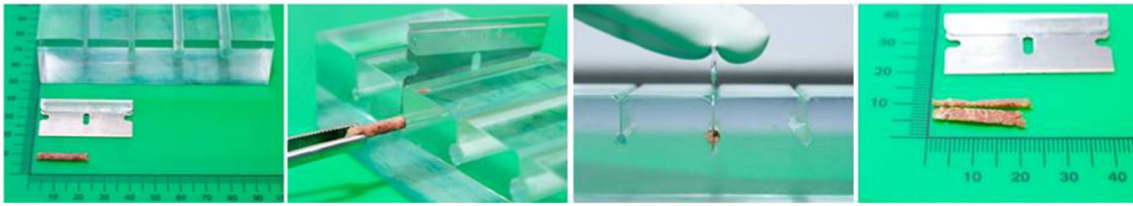
Fig. 1 Splicing of the bone marrow biopsy in a Perspex mold
