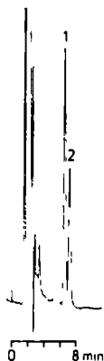
Fig 5 Chromatogram of dog urine sample taken after intravenous administration of NPFA (0.9 mg/kg) containing 3.7 mg/l NPFA. Peaks. 1 = NPFA; 2 = unknown metabolite.
