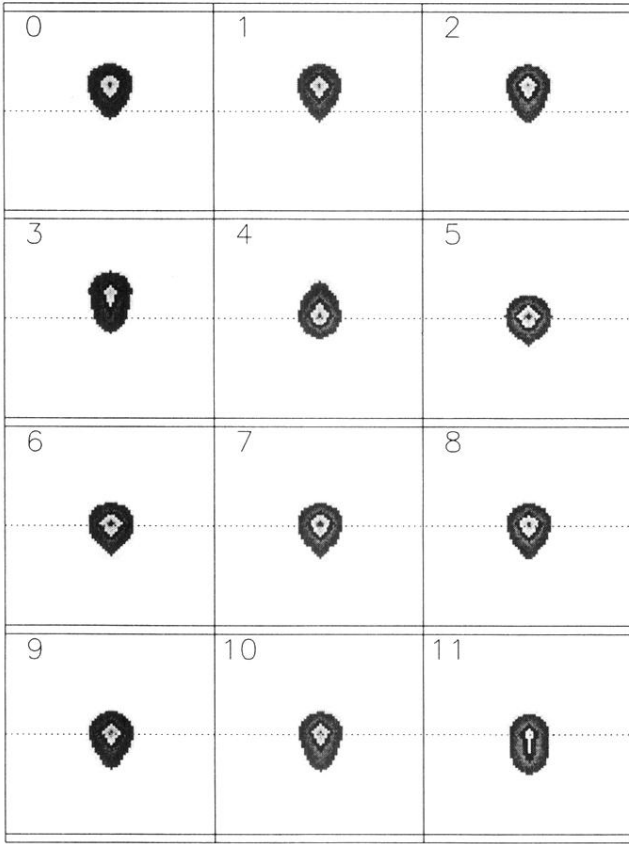
FIG. 7. Snapshots of a smooth interpolation of one vortex current vorticity distribution in an 8 \times 8 sublattice of a 16 \times 16 array, for two different current values: (a) i_b = 0.11 , (b) i_b = 0.60 . Different gray scales represent different levels of current vorticity. In the first snapshots (labeled as 0), the black dot is the middle point of the vortex. The dashed line (fixed in time) is a guide to the eye. In (a) the time interval between two snapshots is \Delta t = 10 (in units of 1/\omega_c ). The vortex moves over one plaquette in approximately t = 7\Delta t . In (b) the time interval between successive snapshots is \Delta t = 0.625 in units of 1/\omega_c , and here the period of the motion is approximately t = 4.5\Delta t .
