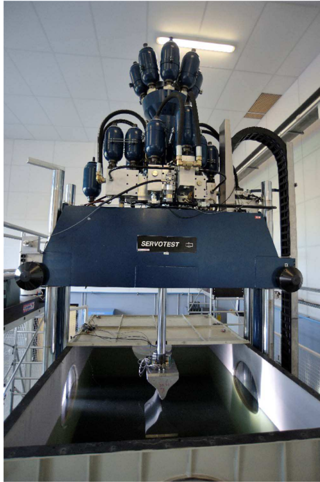
Fig. 13. The hydraulic shock machine used for the experimental impact tests. The water tank is underneath the shock machine. The cone is not shown on this picture.
