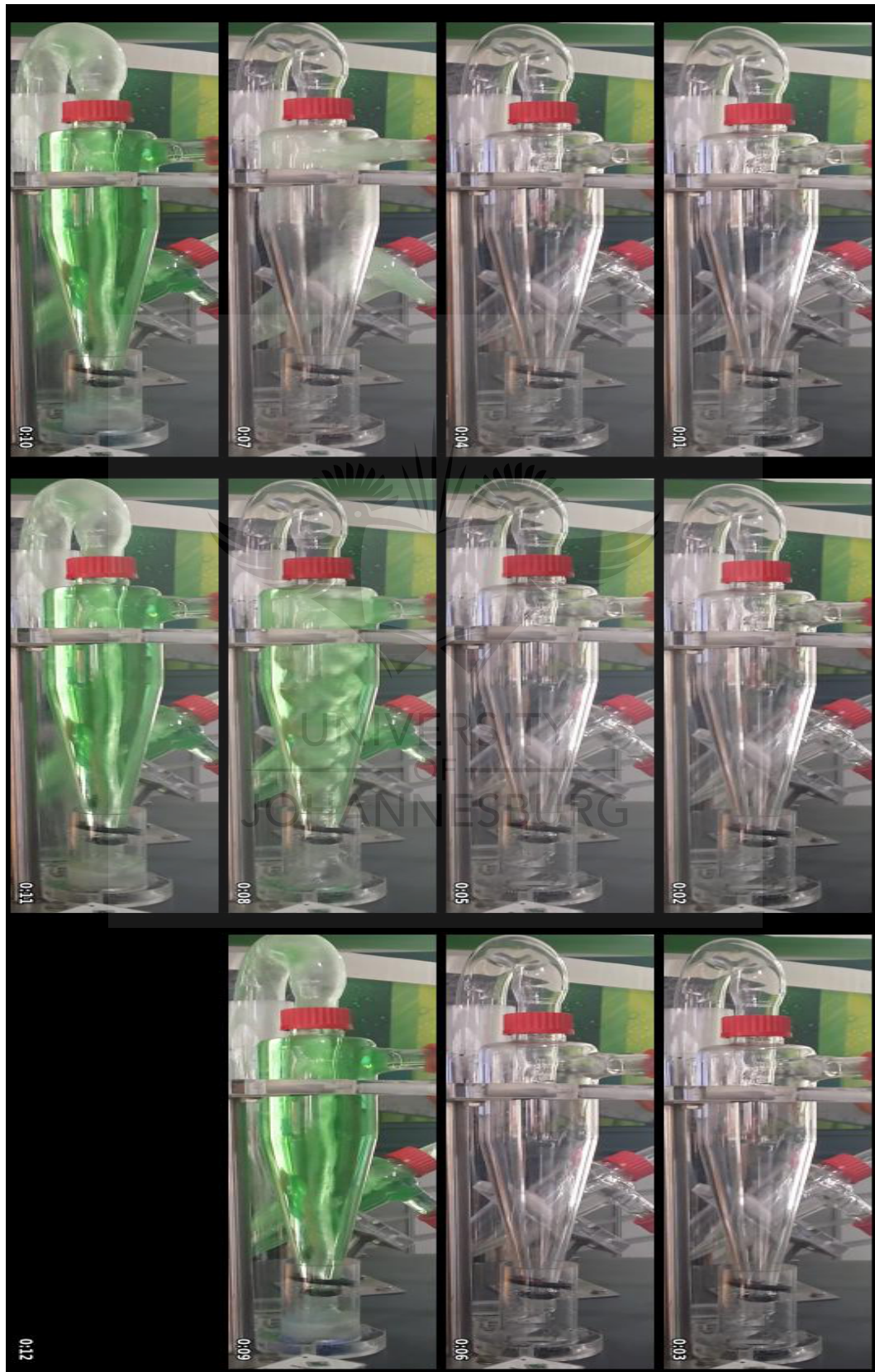
Figure 5.14: Image stills from video of air-core formation with dye
