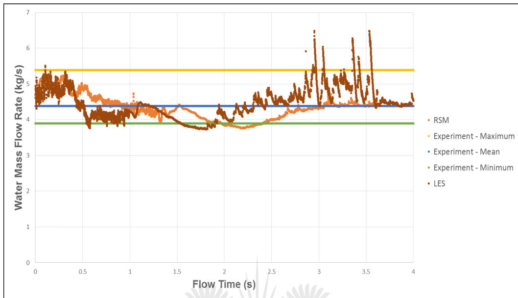
Figure 6.35: Overflow water mass flow rate as predicted by the NS based VOF-DEM models
