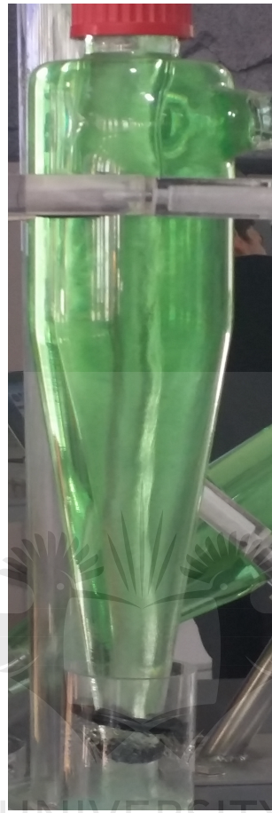
Figure 6.2: Air-core in perspex half scale hydrocyclone - green dye added to reveal air-core
