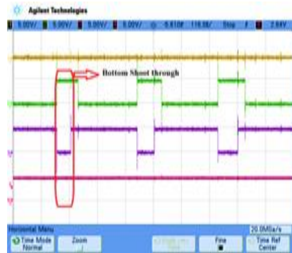
Figure 9. Gate pulses of one leg in bottom shoot through
