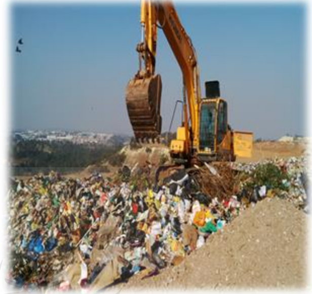
Excavator mixing wastes before sampling
