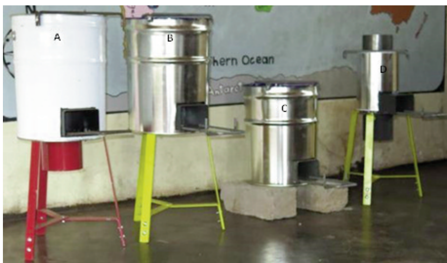
Figure 3: The Tshulu stoves: (A) Tshulu2 with ash remover; (B and C) RS1 and RS2 based on the Aprovecho designs; (D) the smaller design Tshulu1.
