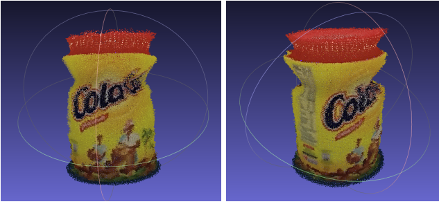
Fig. 13 64 point clouds aligned with ICP after applying all the noise removal operations, translation and rotation. Front view (left) and perspective (right).
