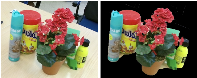
Fig. 16 RGB image of a sample scene (left), and the same image after GrabCut segmentation (right).
