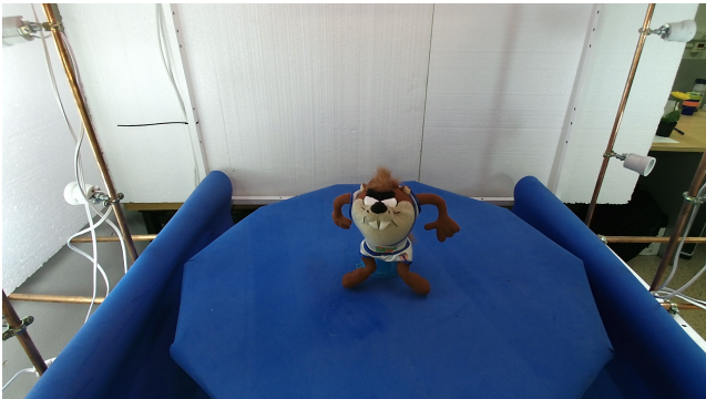
Fig. 2 Our turntable with an object placed near its center, note the blue color of the platform to perform chroma keying operations.
