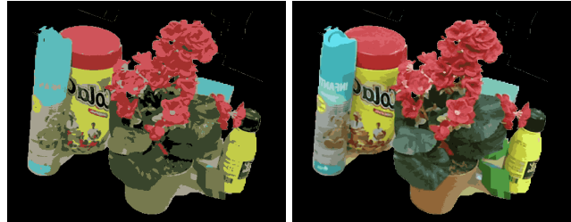
Fig. 17 Segmented scene after color quantization with 8 clusters (left), and after quantization with 48 clusters (right).
