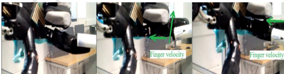
Figure 9: Experiment with the servo-tactile control. Controlling magnitude and position of the force in the contact.
