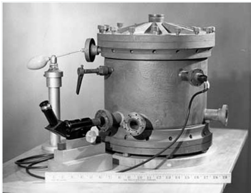
Original apparatus used by Millikan in his oil-drop experiment. Credits: Wikipedia .
