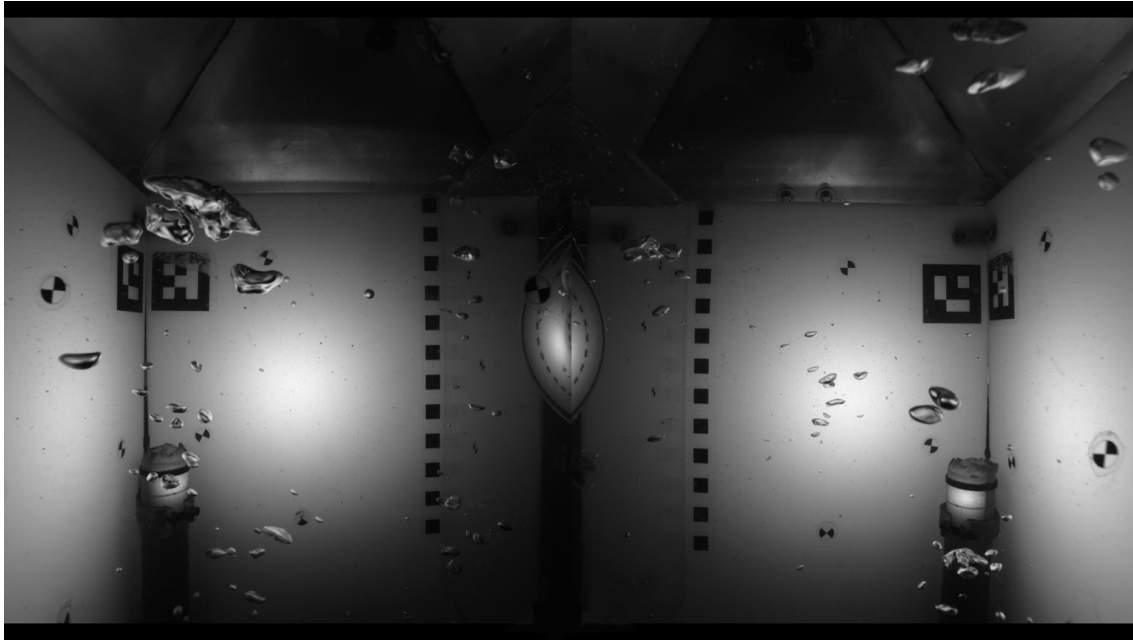
Fig. 21: Bubble Box above Bubble Catcher vent (ca. 250 ml/min). The two images left (bubble 1') and right (bubble 2') are synchronized and have been taken at exactly the same time.
