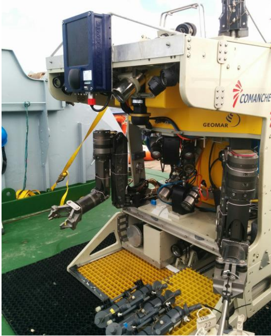
Fig. 28: Picture of the ROV PHOCA equipped with the CODAECHOSCOPE sonar.
