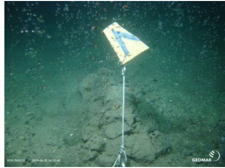
Fig. 3b: First Marker set for later Bubble Catcher deployment within the crater at a seep field consisting of minor to major vent sites.
