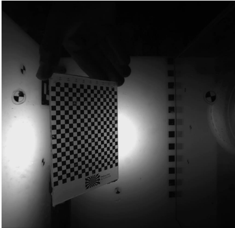
Fig. 30: Checkerboard calibration before deployment.
