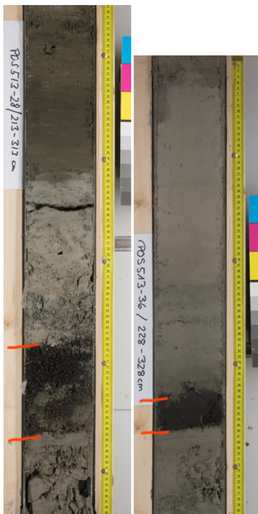
Fig. 1: The black lapilli layer (left) and the black ash layer (right) lie at the same depth below seafloor but 45 km apart. This seems to be a mafic fallout that thickens and coarsens toward Santorini.
