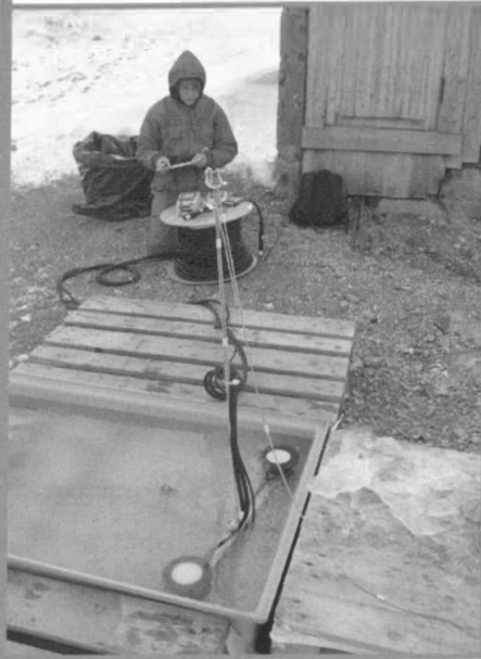
Figure 9 UV radiation measurements in the experiment tank. Sensor detection unit is in the foreground (tank), data logging equipment triggered by a scientist is in the background.
