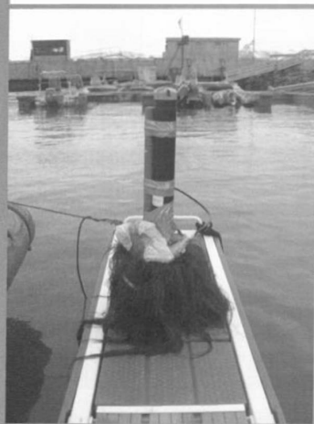
Figure 6 ADCP mounted on a heavy concrete bucket (with attached algae after overnight deployment).
