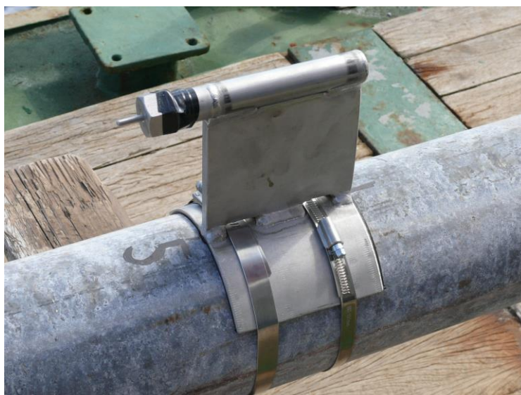
Figure 21 MTL mounted on the gravity corer on cruise P472. The pointy end with the thermistor is facing downward.
