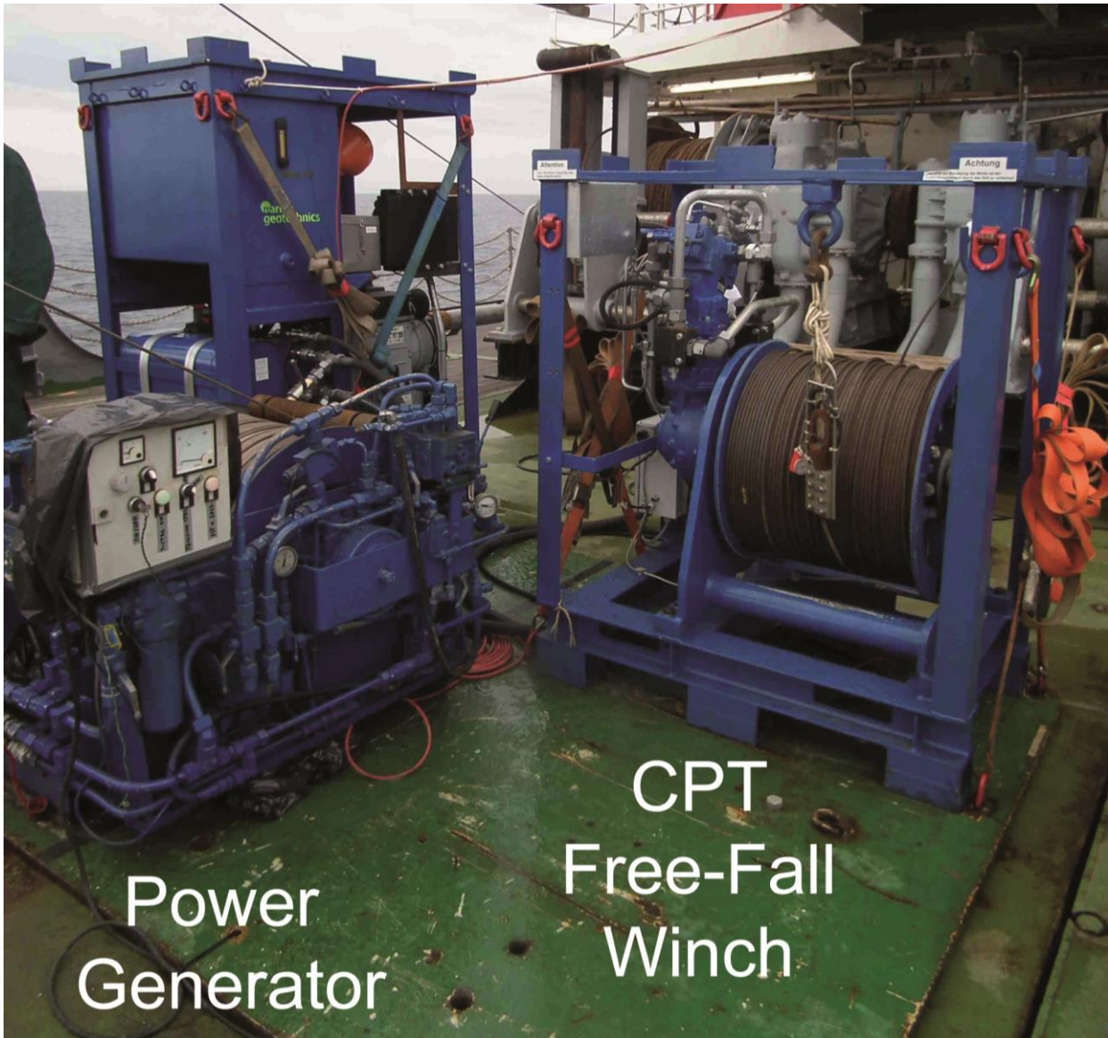
Figure 12 New MARUM FF-CPTu-Winch 200 m (left) and entire assembly together with hydraulic aggregate (right).
