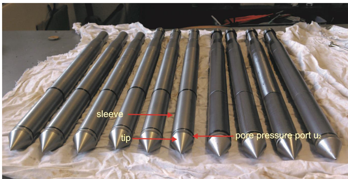
Figure 9 Digital pressure-compensated compression CPTu cones, as installed in the GOST system.
