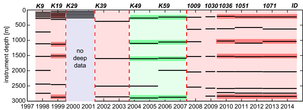
Figure 7. Selection of current meter levels from full-coverage array (red) for transports regressed from single mooring coverage (green). Mooring IDs for the central mooring K9 (see also timeline in Figure 2) are listed at the top. The gray-shaded mooring K29 (1999–2001) yielded only ADCP data above 300 m.
