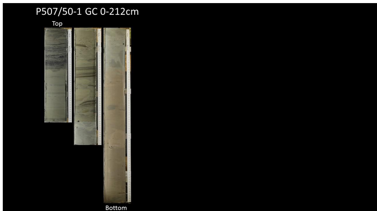
Fig. 4.3-9: Core photos of the uppermost 2 m of the sediment core 50-1 from the southern part of the Landsort Deep documenting a succession of several Holocene mass wasting events.
